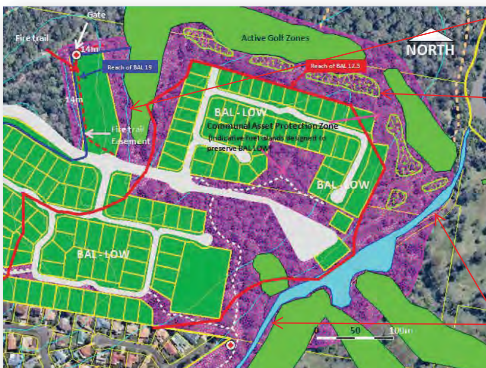
Figure 12. Fire trail protection zone provides for a safer fire trail and sufficient setback for viability of BAL 12.5. (Protection Zone widths noted in metres).
