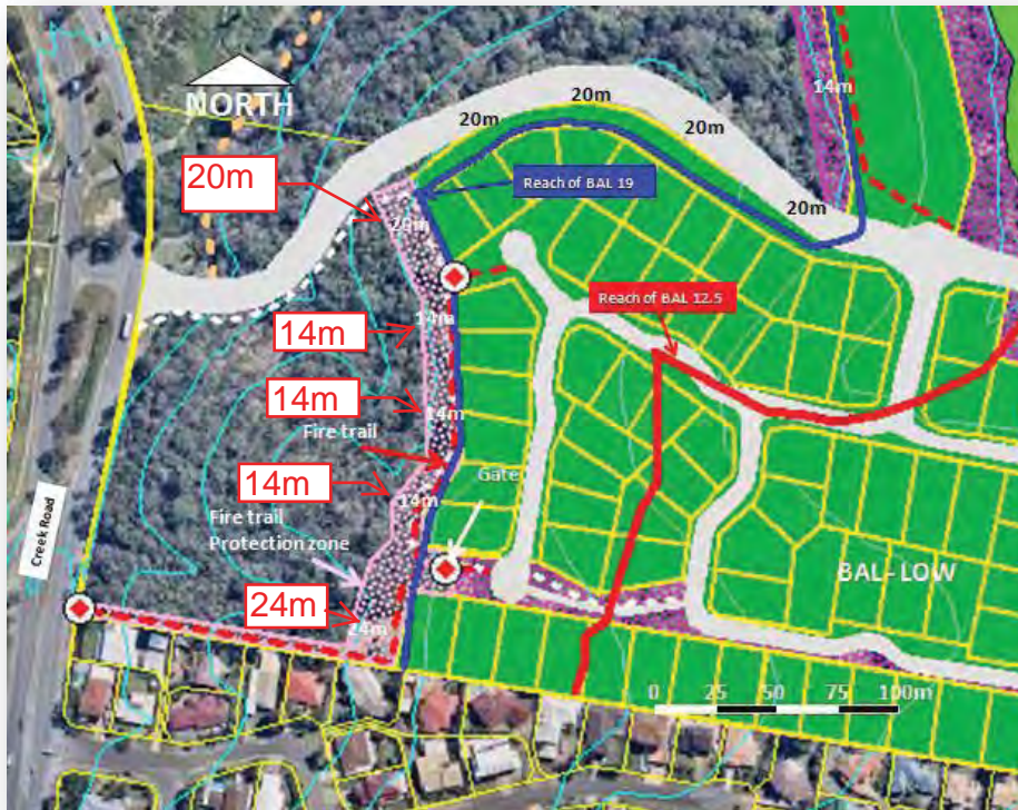
Figure 12. Fire trail protection zone provides for a safer fire trail and sufficient setback for viability of BAL 12.5. (Protection Zone widths noted in metres).
