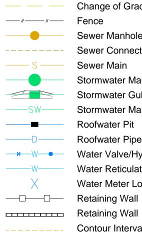
Change of Grade Sewer Manhole Sewer Connection Sewer Main Stormwater Manhole Stormwater Gully Pit Stormwater Main Roofwater Pit Roofwater Pipe Water Valve/Hydrant Water Reticulation Water Meter Location Contour Interval 0.5m
